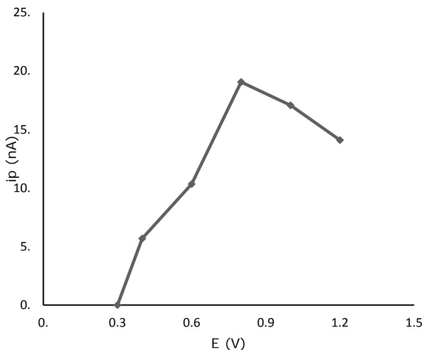
**Fig. 3.** Hydrodynamic voltammogram for 250  $\mu\text{M}$  serotonin. Conditions: running buffer: 20 mM MES-NaOH pH=7.0; separation voltage=1000 V, and injection voltage=750 V for 3 s
