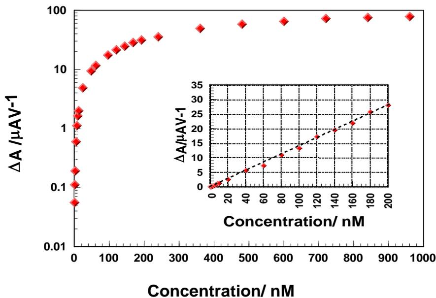
**Fig. 8.** The calibration curve for acrylamide standard solutions in the range of 0.01 nM to 800 nM the inset shows the linear relationship between  $\Delta A$  and  $\log(C)$  (nM) in the range of 0.1 nM to 200 nM, Inset voltammogram
