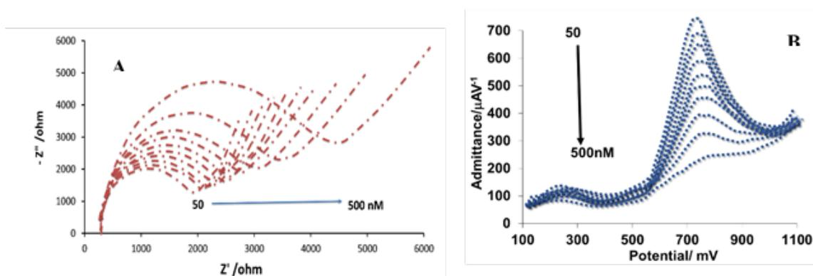
**Fig. 5.** EIS at ssDNA/AuNPs/PANI-CHI/Au before and after incubation with different acrylamide (50–500 nM) in 100 M KCl, 100 mM PBS pH 7.5 solution, applying a sinusoidal AC waveform of 10 mV in amplitude at the frequency range 1–1000 Hz. Experimental admittance of the solution under same condition at SW frequency 500 Hz and amplitude 25 mV
