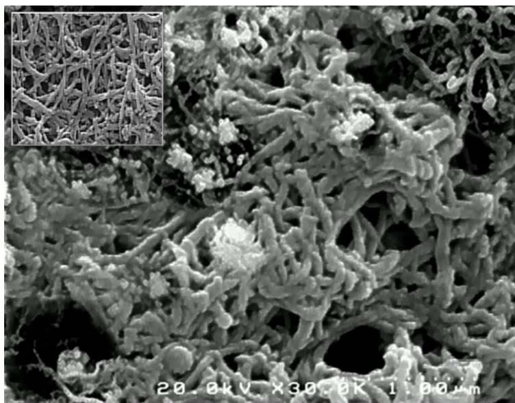
**Fig. 3.** SEM image of Au NPs/PANI/Au, the inset (PANI-CHI/Au)
