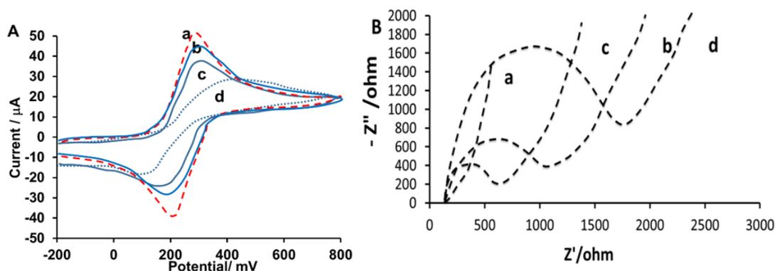
**Fig. 4.** A) Cyclic voltammograms of (a) bare Au, (b) PANI-CHI/Au, (c) Au NPs/PANI-CHI/Au, (d) ssDNA/Au NPs/PANI-CHI/Au, electrodes in PBS solution, pH 7.5, Scan rate  $50 \text{ mV/s}^{-1}$ ; B) EIS plots of (a) bare Au, (b) PANI-CHI/Au, (c) Au NPs/PANI-CHI/Au, (d) ssDNA/Au NPs/PANI-CHI/Au, electrodes in 100 mM PBS solution, pH 7.5,  $[\text{Fe}(\text{CN})_6]^{3-/4-}$  3mM, Frequency range 0.1 Hz to 1 MHz, DC potential of 200 mV and AC amplitude of 10 mV.
