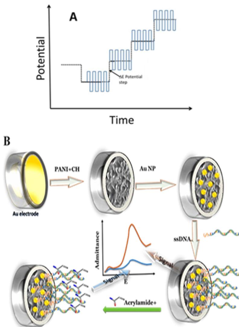
**Fig. 2.** Schematic presentation of A) the applied potential waveform for FFTAV measurement; B) biosensor fabrication
