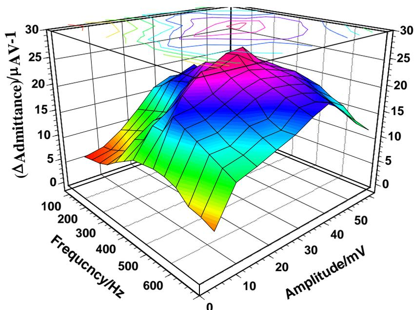
**Fig. 6.** The effect of frequency and amplitude on the response of the ssDNA/AuNPs/PANI-CHI/Au in  $1.0 \times 10^{-7}$  M acrylamide in 100 M KCl, 100 mM PBS pH 7.5 solution
