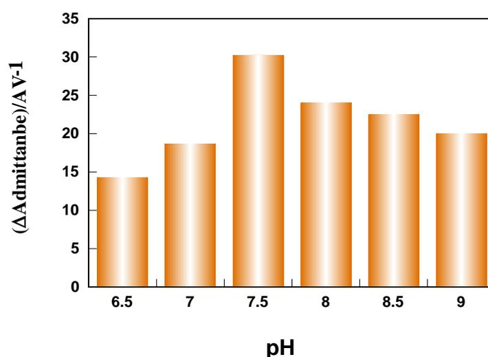
**Fig. 7.** The effect of pH on the response of the biosensor in solution of  $1.0 \times 10^{-7}$  M Acrylamide 100 mM KCl and 100 mM PBS. The SW frequency was 300 Hz at amplitude 25 mV
