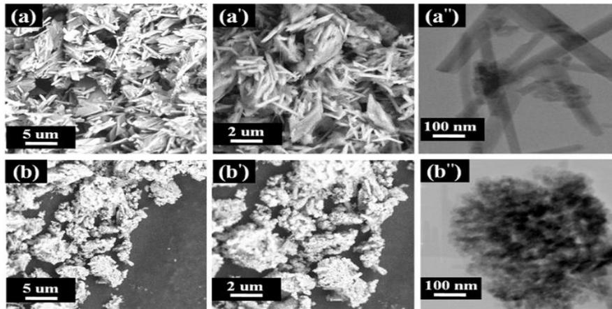
**Fig. 2.** FE-SEM and TEM micrographs of (a, a' and a'') oxalate precursor and (b, b' and b'') NS-LMNCO
