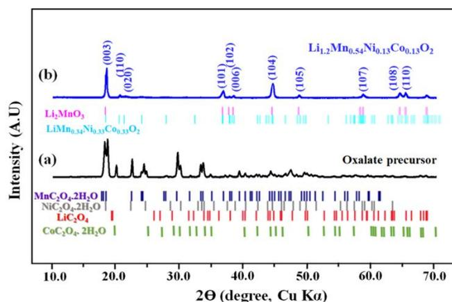
**Fig. 1.** XRD patterns of (a) oxalate precursor and (b) Nano sponge  $\text{Li}_{1.2}\text{Mn}_{0.54}\text{Ni}_{0.13}\text{Co}_{0.13}\text{O}_2$  (NS-LMNCO)
