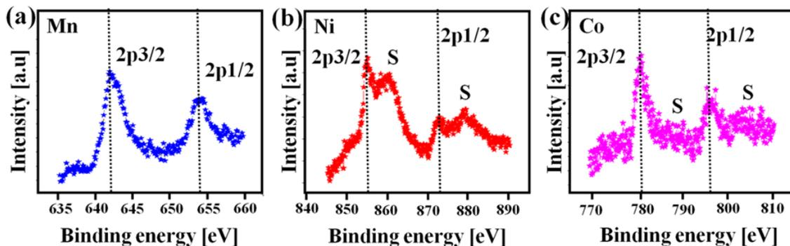
**Fig. 3.** X-ray photoelectron spectroscopy (XPS) of Mn (a), Ni (b) and Co (c) for NS-LMNCO
