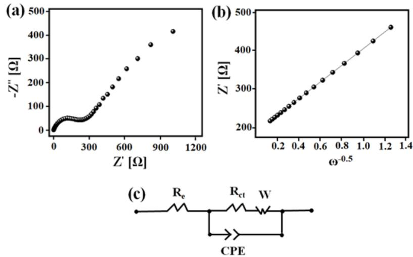
**Fig. 5.** (a) Nyquist plot, (b) Warburg factor determination plot of NS-LMNCO electrode at low frequencies and (c) equivalent circuit model. The double layer and passivation film capacitances are assigned by CPE
