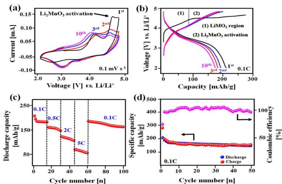
**Fig. 4.** (a) Cyclic voltammograms and (b) charge and discharge profiles of NS-LMNCO sample between 2 and 4.8 V recorded at a scan rate of  $0.1 \text{ mV s}^{-1}$  and  $0.1 \text{ C}$ , respectively. (c) Rate capacities of NS-LMNCO electrode at  $0.1\text{C}$  to  $5 \text{ C}$ . (d) Cycling performance of NS-LMNCO at  $0.1 \text{ C}$  for 50 cycle
