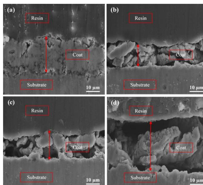
**Fig. 4.** Cross-section SEM micrographs of 6061 Al alloy with PEO coatings: (a)  $10 \text{ g L}^{-1}$   $\text{NaAlO}_2$ ; (b)  $12 \text{ g L}^{-1}$   $\text{NaAlO}_2$ ; (c)  $14 \text{ g L}^{-1}$   $\text{NaAlO}_2$  and (d)  $16 \text{ g L}^{-1}$   $\text{NaAlO}_2$  at magnification of 1000x
