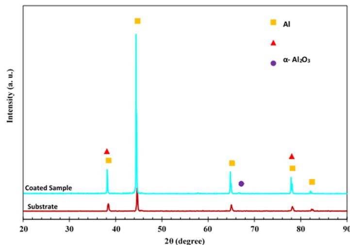
**Fig. 5.** X-ray diffraction patterns of 6061 Al alloy with and without PEO coating.
