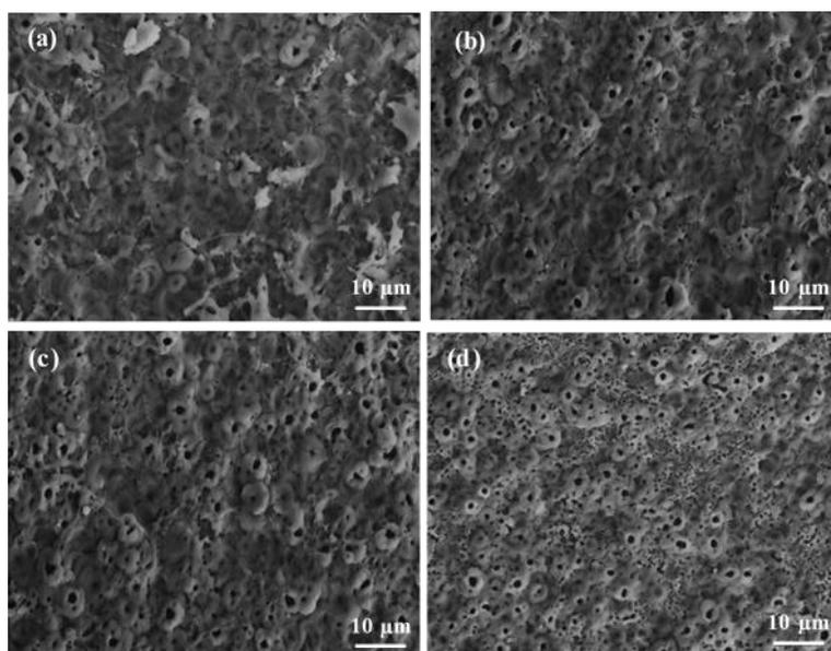
**Fig. 3.** SEM micrographs of 6061 Al alloy with PEO coatings: (a)  $10 \text{ g L}^{-1}$   $\text{NaAlO}_2$ ; (b)  $12 \text{ g L}^{-1}$   $\text{NaAlO}_2$ ; (c)  $14 \text{ g L}^{-1}$   $\text{NaAlO}_2$  and (d)  $16 \text{ g L}^{-1}$   $\text{NaAlO}_2$  at magnification of 1000x
