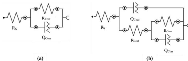
**Fig. 8.** Electrical equivalent circuits used to fit the impedance data of (a) substrate, and (b) PEO coating samples
