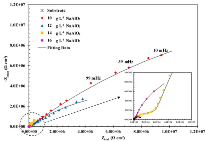
**Fig. 7.** Nyquist plots of PEO coatings on 6061 Al alloy in different concentration of NaAlO<sub>2</sub> in electrolytes
