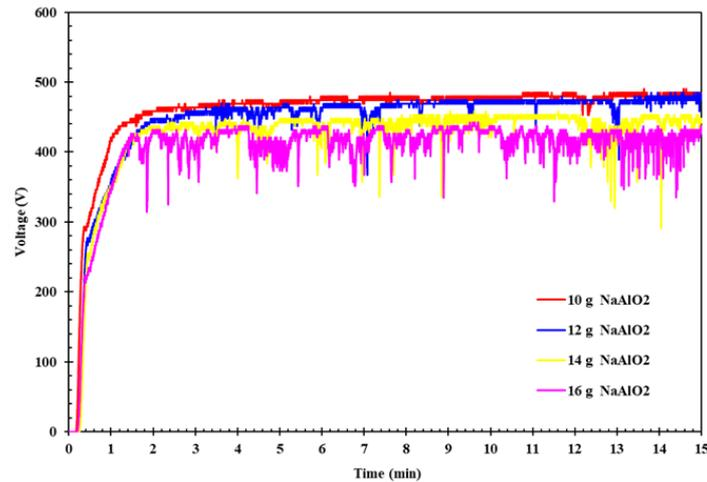
**Fig. 1.** Potential-time curves of PEO coatings on 6061 Al alloy in different concentration of  $\text{NaAlO}_2$  at electrolytes
