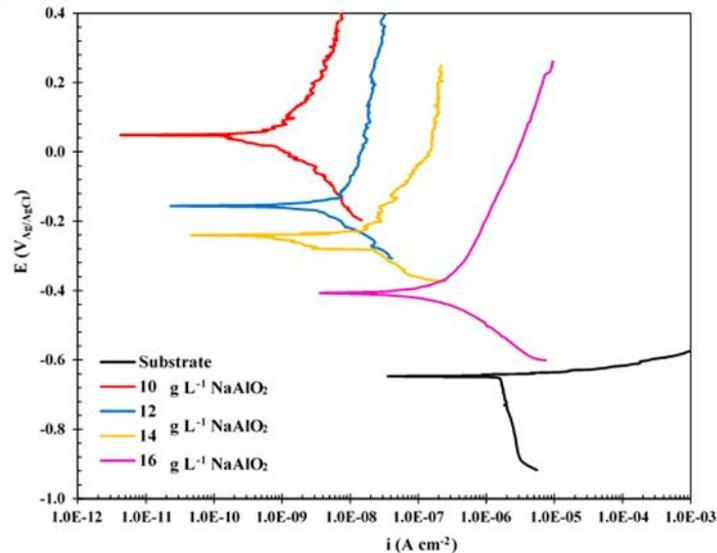
**Fig. 6.** Potentiodynamic polarization plots of PEO coatings on 6061 Al alloy in different concentration of  $\text{NaAlO}_2$  at electrolytes.
