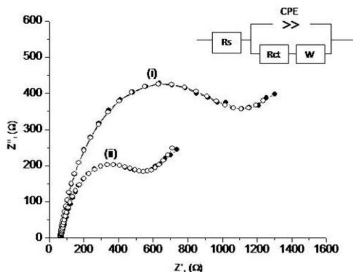
**Fig. 4.** Nyquist plots of a bare (i) and  $\text{CoFe}_2\text{O}_4$  modified (ii) carbon paste electrodes. The experiment was carried out in 5 mM  $[\text{Fe}(\text{CN})_6]^{3-/4-}$ , +210 mV vs. Ag/AgCl, perturbation amplitude: 5 mV pp, frequency range: 50 kHz to 10Hz). The inset is the Randels equivalent circuit. The charge transfer resistance at the bare electrode is  $1005 \Omega$  and at the modified electrode is  $473 \Omega$ . The open symbols are the fitted values
