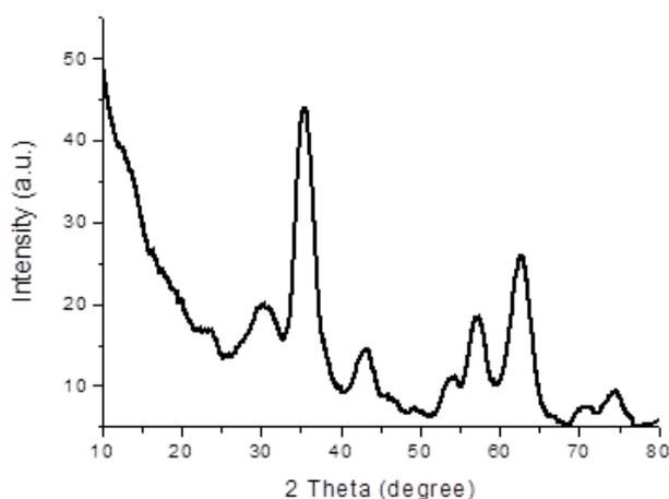
**Fig. 2.** X-ray diffraction (XRD) pattern of cubic  $\text{CoFe}_2\text{O}_4$  nanoparticles prepared by coprecipitation of Co and Fe precursors in basic medium
