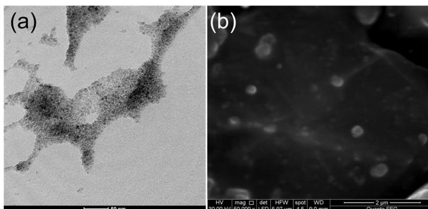
**Fig. 1.** (a) Transmission electron microscopy (TEM) image of  $\text{CoFe}_2\text{O}_4$  NPs prepared using Co and Fe precursors in basic medium, spherical in shape with approximately size 7.0 nm, and (b) Scanning electrochemical microscopy (SEM) micrograph of a carbon paste modified with 5%  $\text{CoFe}_2\text{O}_4$  NPs.
