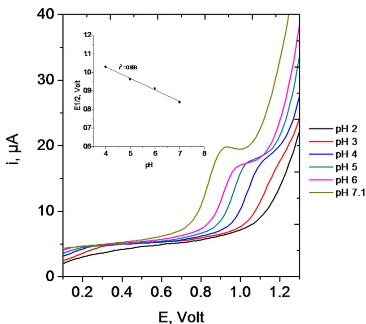
**Fig. 6.** Forward scans of cyclic voltammograms recorded in  $1.0 \times 10^{-4}$  mol/L DON at different pH values using A  $CoFe_2O_4$  modified carbon baste miniaturized electrode; scan rate of 100 mV s. Note: The peak potential is shifted towards negative potential with increasing the pH. A well-shaped with high peak current is observed at pH 7
