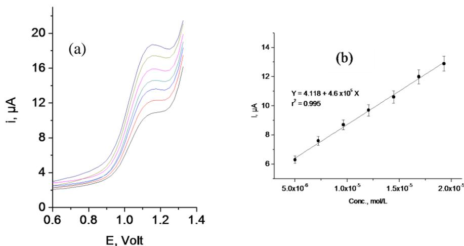
**Fig. 7.** a) Calibration curve using the height  $\Delta i_p$  against  $E$  of anodic DPV peaks at 1.1 mV. Peak heights were determined graphically and plotted against the concentration; b) The corresponding differential pulse voltammograms recorded in a potential range from 0 to +1.4 V *vs.* Ag/AgCl in 0.04 M Britton Robinson buffer (pH=7) with different DON concentrations (5.0–20.0  $\mu\text{mol}$ ) at a  $\text{CoFe}_2\text{O}_4$  modified carbon paste miniaturized electrode
