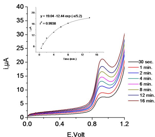
**Fig. 5.** Forward scans of cyclic voltammograms showing the effect of preconcentration time on the sensitivity of the electrode, the experiment was carried out under stirring
