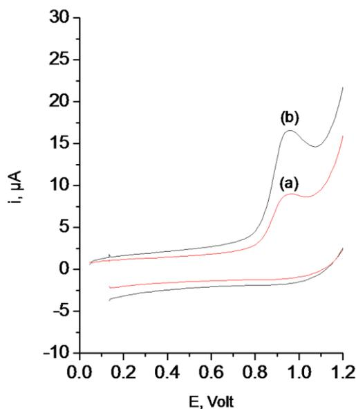
**Fig. 3.** Cyclic voltammogram of (a) a bare and (b) modified carbon paste electrodes of  $1 \times 10^{-5}$  mol/L donepezil HCl in Britton Robinson buffer pH 7
