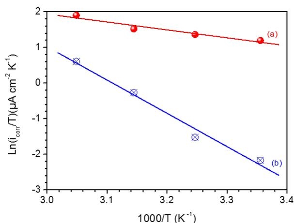
**Fig. 7.** Transient Arrhenius plot for mild steel in 1 M HCl in the absence and presence of  $10^{-3}$  M PID at different temperatures
