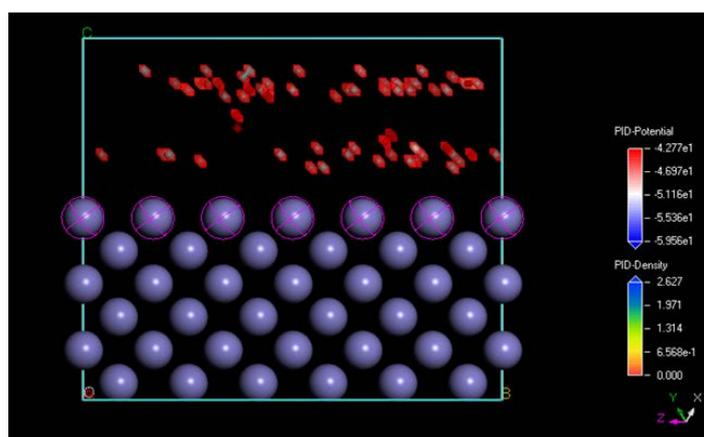
**Fig. 13.** Adsorption density field for Fe (110)/PID interface obtained through the Monte Carlo simulation
