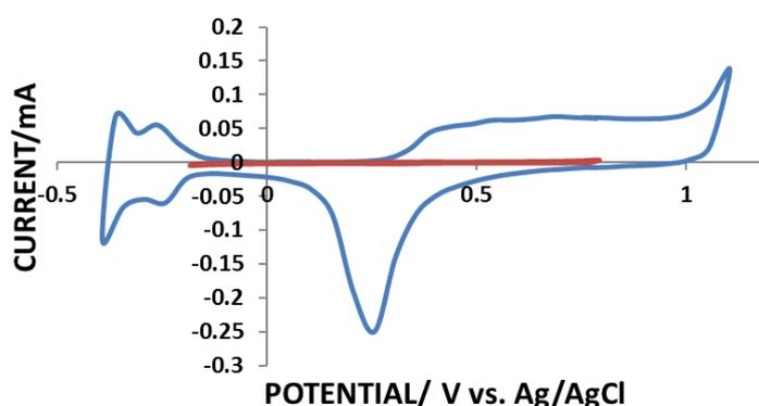
**Fig. 1.** The cyclic voltammogram of (A) polycrystalline platinum electrode and (B) the same electrode after adsorption of iodine from 0.50 M+ $1.0 \times 10^{-2}$  M KI solution. Both i-E scans were recorded in iodine-free 0.5 M H<sub>2</sub>SO<sub>4</sub> at a scan rate of 50 mV/s
