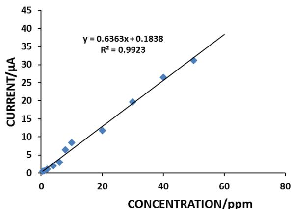
**Fig. 3.** An extended calibration curve shows the relationship between Fe(II) concentration and the anodic peak current measured from the voltammograms for Fe(II) in 0.50 M H<sub>2</sub>SO<sub>4</sub> at iodine-coated platinum electrode. Scan rate=50 mV/s
