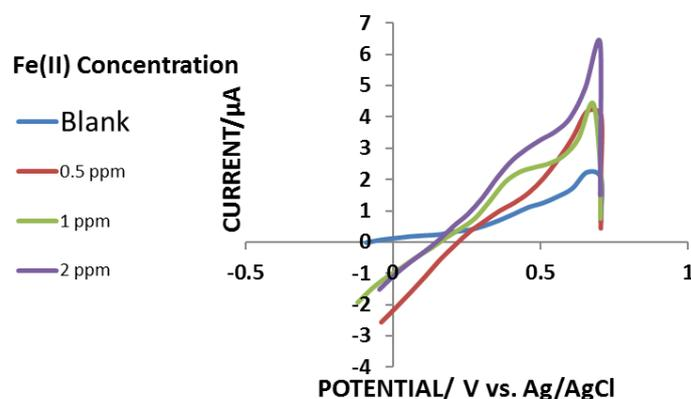
**Fig. 2.** The cyclic voltammogram of iodine –coated electrode recorded in 0.5 M H<sub>2</sub>SO<sub>4</sub> solution containing: (—) blank, (—) 0.5 ppm Fe(II), (—) 1 ppm Fe(II), and (—) 2 ppm Fe(II). Scan rate=50 mV/sec
