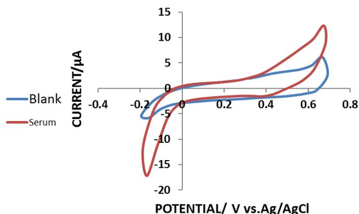
**Fig. 4.** Cyclic voltammograms of an iodine-coated platinum electrode in human blood serum sample after the treatment with 1 M HNO<sub>3</sub> and a few crystals of hydroxylamine
