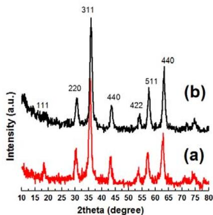
**Fig. 1.** XRD patterns of the electro-synthesized (a) pristine  $\text{Fe}_3\text{O}_4$  and (b)  $\text{Fe}_3\text{O}_4/\text{GO}$  composite
