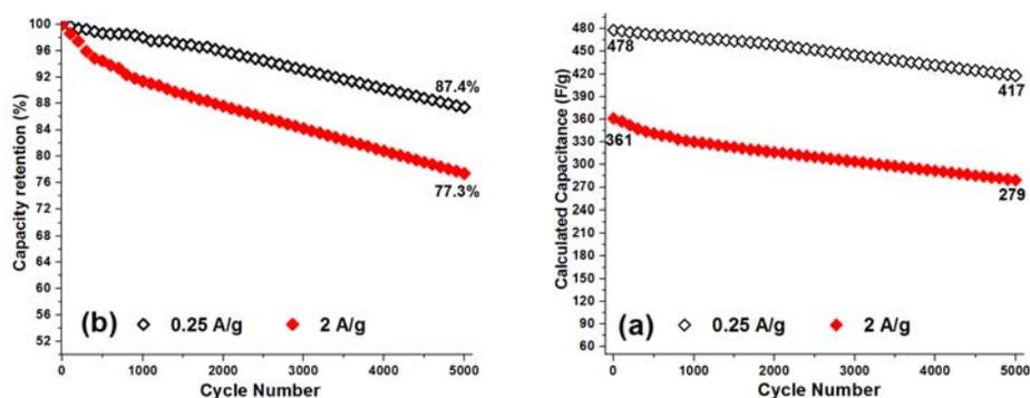
**Fig. 10.** Calculated capacitances and the capacity loss for the fabricated composite during 5000 continuous GCD cycling at the discharge loads of 0.25 and 2 A g<sup>-1</sup>
