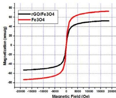
**Fig. 6.** Hysteresis loops for the prepared pristine  $\text{Fe}_3\text{O}_4$  NPs and (b)  $\text{Fe}_3\text{O}_4$  NPs/rGO composite
