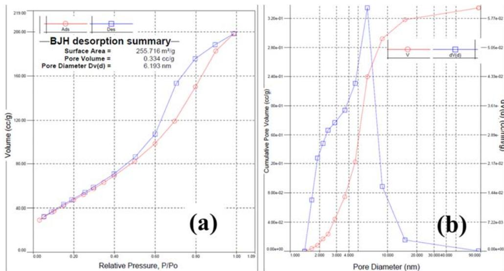
Fig. 7. BET and BJH pore size distribution curves of Fe<sub>3</sub>O<sub>4</sub> NPs/ rGO composite
