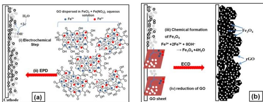
**Fig. 4.** (a,b) Schematic view of the EPD/ECD formation of  $\text{Fe}_3\text{O}_4/\text{rGO}$  composite
