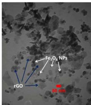
**Fig. 5.** TEM image of the prepared  $\text{Fe}_3\text{O}_4$  NPs/rGO nanocomposite
