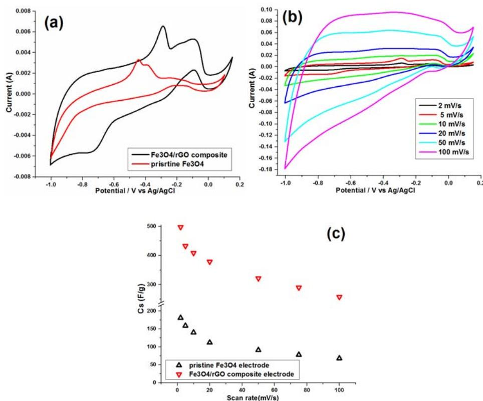
**Fig. 8.** CVs of (a) pristine Fe<sub>3</sub>O<sub>4</sub> NPs and (c,d) Fe<sub>3</sub>O<sub>4</sub> NPs/rGO composite, (c) the calculated Cs values vs. scan rate for both electrodes
