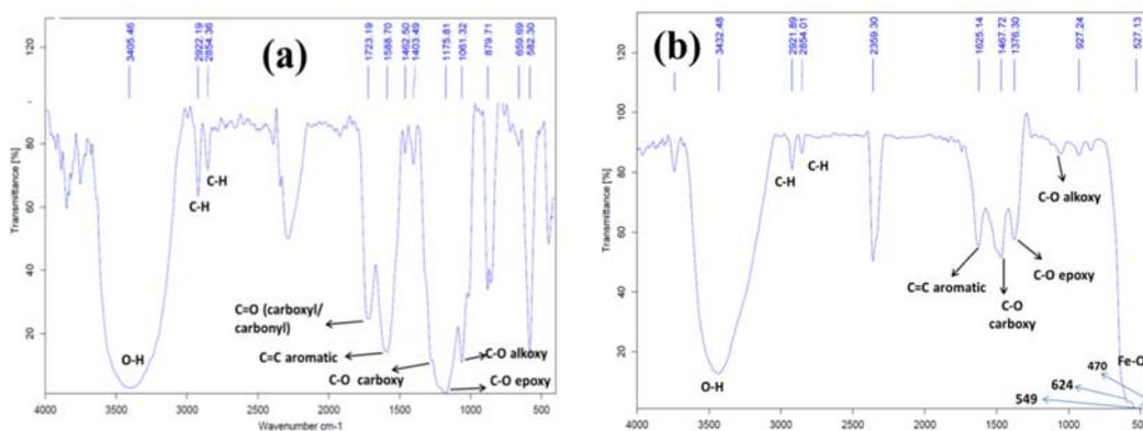
**Fig. 2.** IR spectra of (a) GO and (b)  $\text{Fe}_3\text{O}_4/\text{rGO}$  samples
