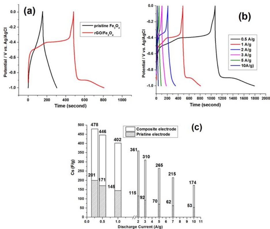
**Fig. 9.** (a) GCD profiles for pristine Fe<sub>3</sub>O<sub>4</sub> and Fe<sub>3</sub>O<sub>4</sub>/rGO electrodes at the current load of 1 A/g and (b) the GCD profiles of Fe<sub>3</sub>O<sub>4</sub>/rGO at various current loads and (c) calculated specific capacity values for both electrodes at the different charge-discharge rates
