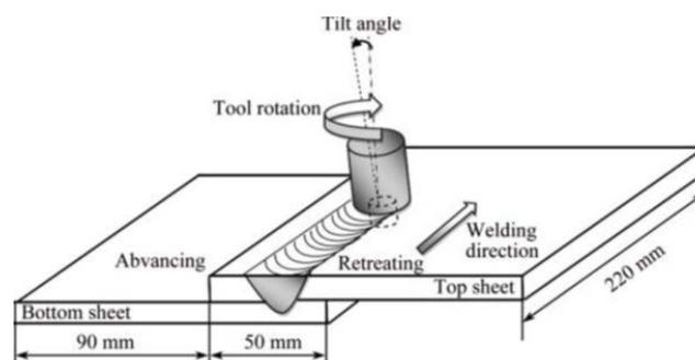
**Fig. 2.** Schematic of friction stir lap welding process and joint design used in this research
