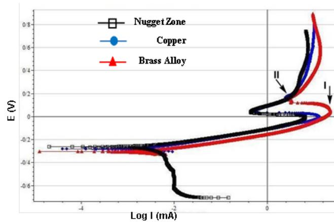
**Fig. 7.** Polarization behavior of Cu, brass alloy and welded copper/brass nugget zone in 1 M NaCl (pH 7.2). Arrows indicate I and II peaks positions
