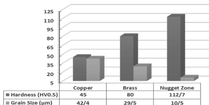
**Fig. 3.** variation of the average Vickers hardness distribution and grain size across the nugget zone (NZ) of welded joint
