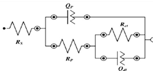
**Fig. 13.** The equivalent circuit utilized for the modeling of EIS data
