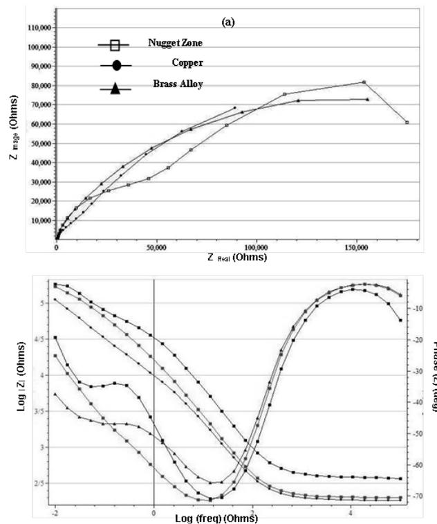
**Fig. 12.** The (a) Nyquist and (b) Bode plots of Cu, brass alloy and welded copper/brass nugget zone in 0.15 M Borax
