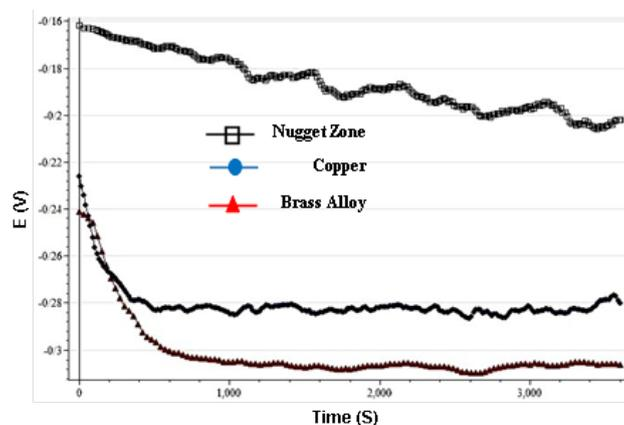
**Fig. 6.** Open circuit measurements for Cu, brass alloy and welded copper/brass nugget zone in 1 M NaCl (pH 7.2) for time duration of 1 h.
