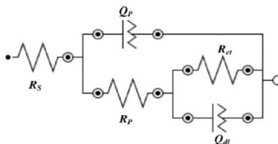
**Fig. 10.** The equivalent circuit utilized for the modeling of EIS data
