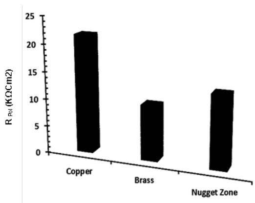
**Fig. 11.** The polarization resistance result from the modeling of experimental EIS data for Cu, brass alloy and welded copper/brass nugget zone in 1 M NaCl
