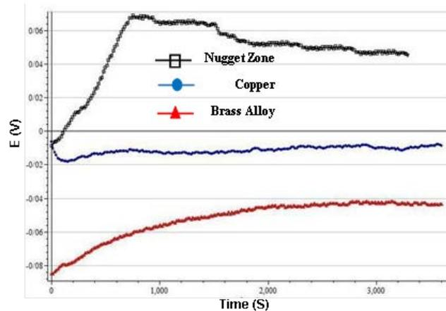
**Fig. 5.** Measurements of Cu open circuit, brass alloy and welded copper/brass nugget zone in 0.015 M Borax (pH 9.3) for 1 h
