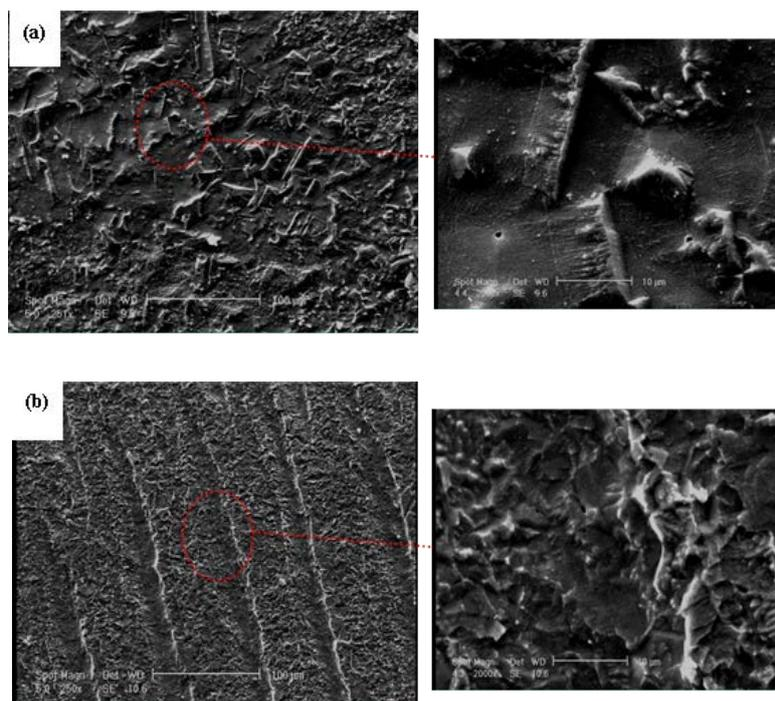
**Fig. 14.** SEM micrographs for the WNZ surfaces formed in solutions of various pH (a) pH 7.2 (b) pH 9.3
