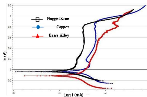
**Fig. 8.** Polarization behavior of Cu, brass alloy and welded copper/brass nugget zone in 0.015 M Borax (pH 9.3)
