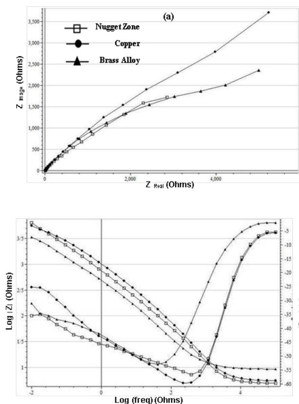
**Fig. 9.** (a) Nyquist plot (b) Bode plot for Cu, Brass alloy and welded copper/brass nugget zone in 1 M NaCl
