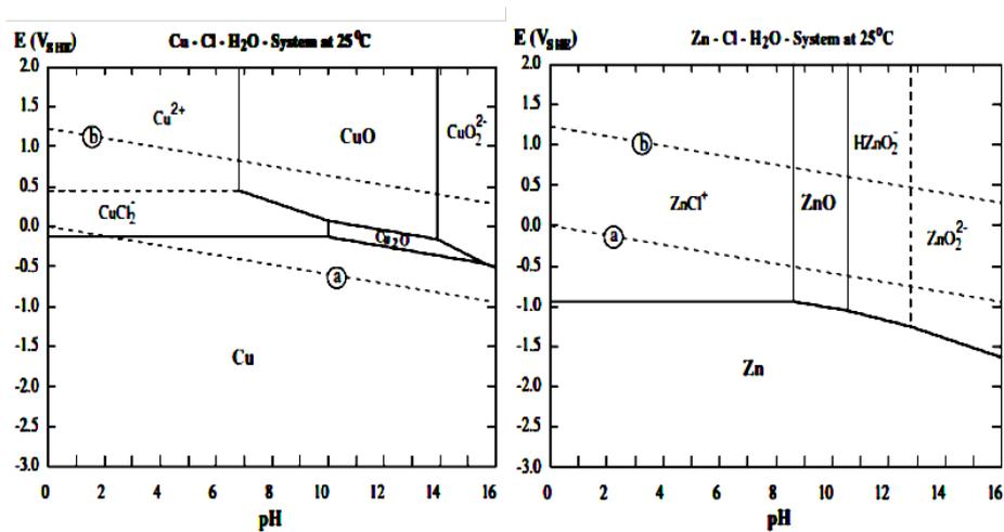
**Fig. 4.** Pourbaix diagrams of Cu and Zn in Cl<sup>-</sup>-H<sub>2</sub>O system at 25 degrees at 0.67 activity of Cl<sup>-</sup>, equal to 1 M of NaCl [24]
