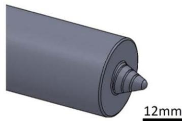
**Fig. 1.** shape of the welding tool designed in experiment
