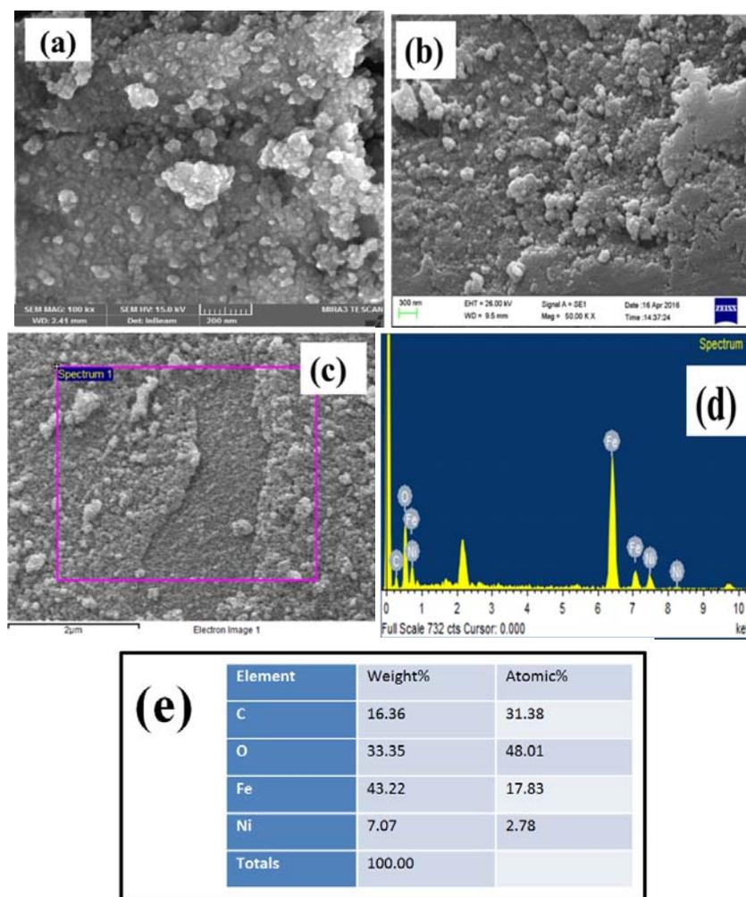
**Fig. 2.** FE-SEM images of (a) pure Ni doped iron oxide and (b,c) its composite with GO, and (d) EDS graph and (e) the elemental percentages in the composition of prepared sample
