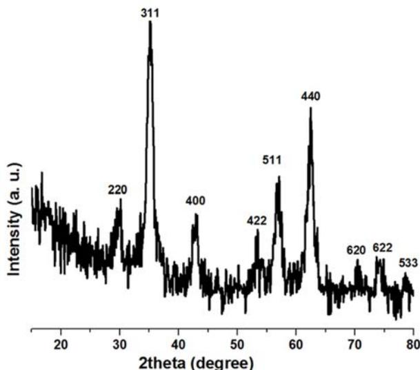
**Fig. 1.** XRD pattern of the prepared metal ion doped iron oxide/GO composite
