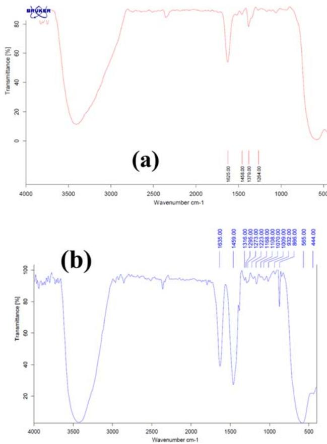
**Fig. 3.** IR spectra of the synthesized (a) pure Ni doped iron oxide and (b) its composite with GO
