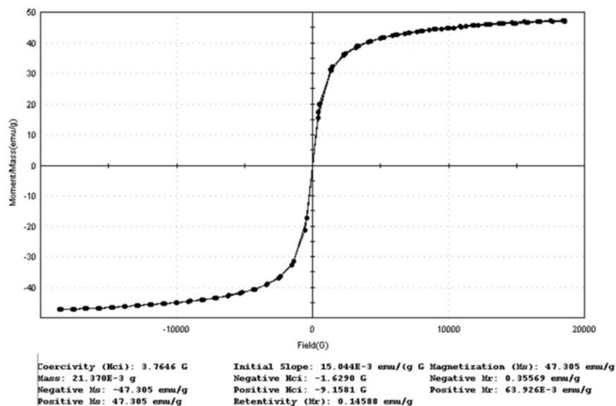
**Fig. 4.** Magnetization curve obtained by vibrating sample magnetometer (VSM) analysis at room temperature
