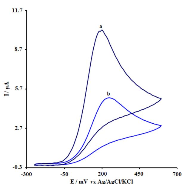
**Fig. 5.** Cyclic voltammograms of (a) Ag(I)/SPE and (b) bare SPE in 0.1 M PBS (pH 7.0) in the presence of 200.0  $\mu\text{M}$  norepinephrine at the scan rate  $50 \text{ mVs}^{-1}$
