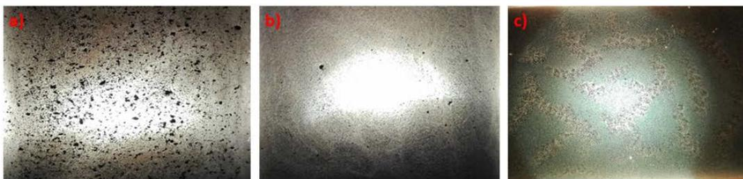
**Fig. 3.** Coatings containing PANI with different DBSA content. DBSA 0 (a); DBSA 1 (b) and DBSA 3 (c)
